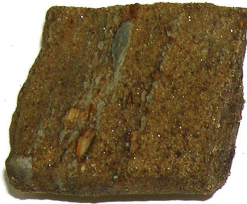
Figure 5-11: Sandstone Core From Outside of Petroleum-Impacted Zone Showing Orange to Red Coloring, Which Indicates High Iron Content and Oxidizing Ground Water Conditions
